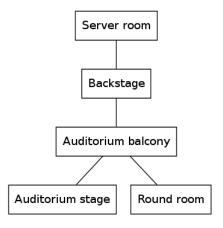
This network was unmanaged gigabit throughout. We tested point-to-point connections between machines with iperf, and saw performance of ~930 Mbps for unidirectional TCP streams.
